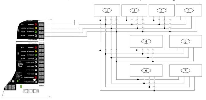
Figure 3.6: SDI2 Devices System Wiring Diagram
